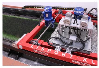
Replicates compaction found in real condition
