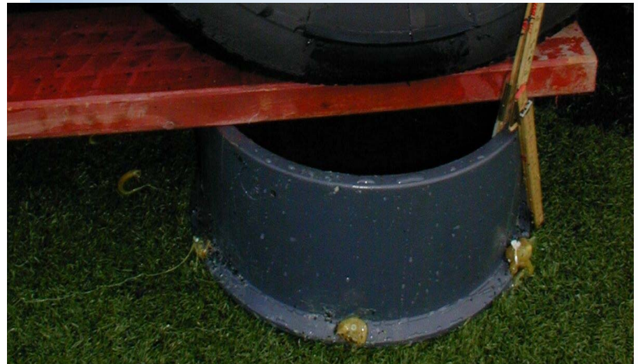
Photo: The cylinder is pressed onto the surface by using the weight of the car
