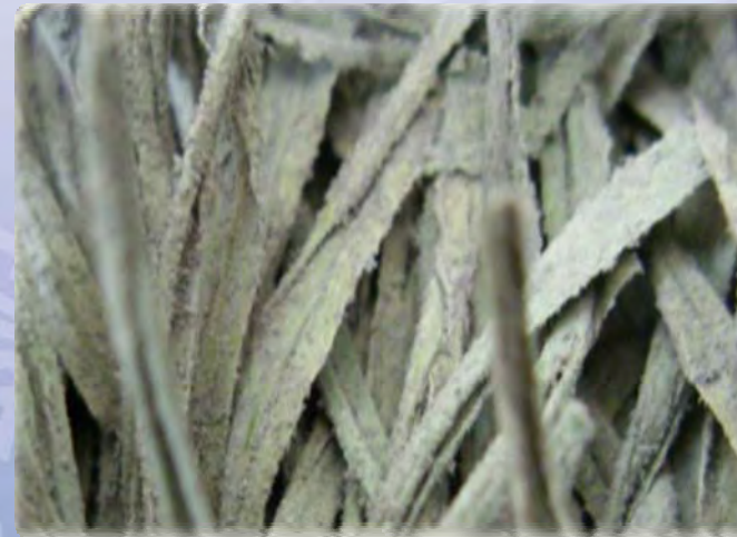
Filled with 6 %wt nano SiO 2
