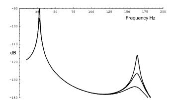
The rationale for a filter with cut-off at 120 Hz appears to be to eliminate the signal from the secondary peak. However, the intensity of the secondary peak is 35 to 50 dB below that of the main peak. So the 120 Hz filter with a reasonably steep cut-off, say 4 pole at 24 dB/Octave, would produce a 6 to14 dB attenuation at the frequencies of the secondary peak, thus reducing the energy leakage from this peak to about 0.1 to 1
