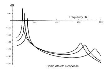
The three curves represent the responses for surfaces with Force Reductions of 50, 40 and 30 % (from left to right). The primary peak below 50 Hz is due to the vibration of the 20 kg mass, and the secondary peak, at 155 to 200 Hz, to the vibration of the 3 kg foot. (It would be 7 % lower in frequency for a 3.5 kg foot) The concrete response would be a single peak at 50 Hz.
