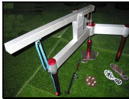
Figure 1. Rotational resistance apparatus
