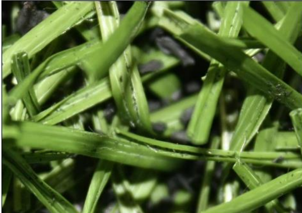
Competitor after 30 000 Cycles in the Lisport test, produced in the middle east
