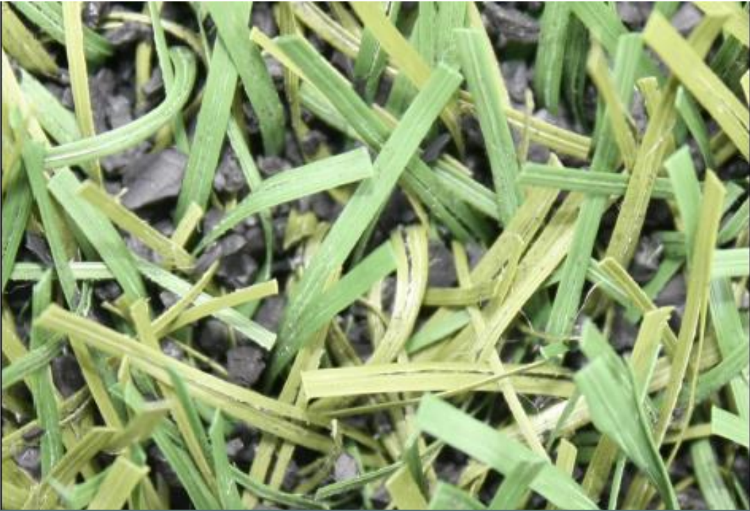
Competitor after 30 000 Cycles in the Lisport test, produced in Spain
