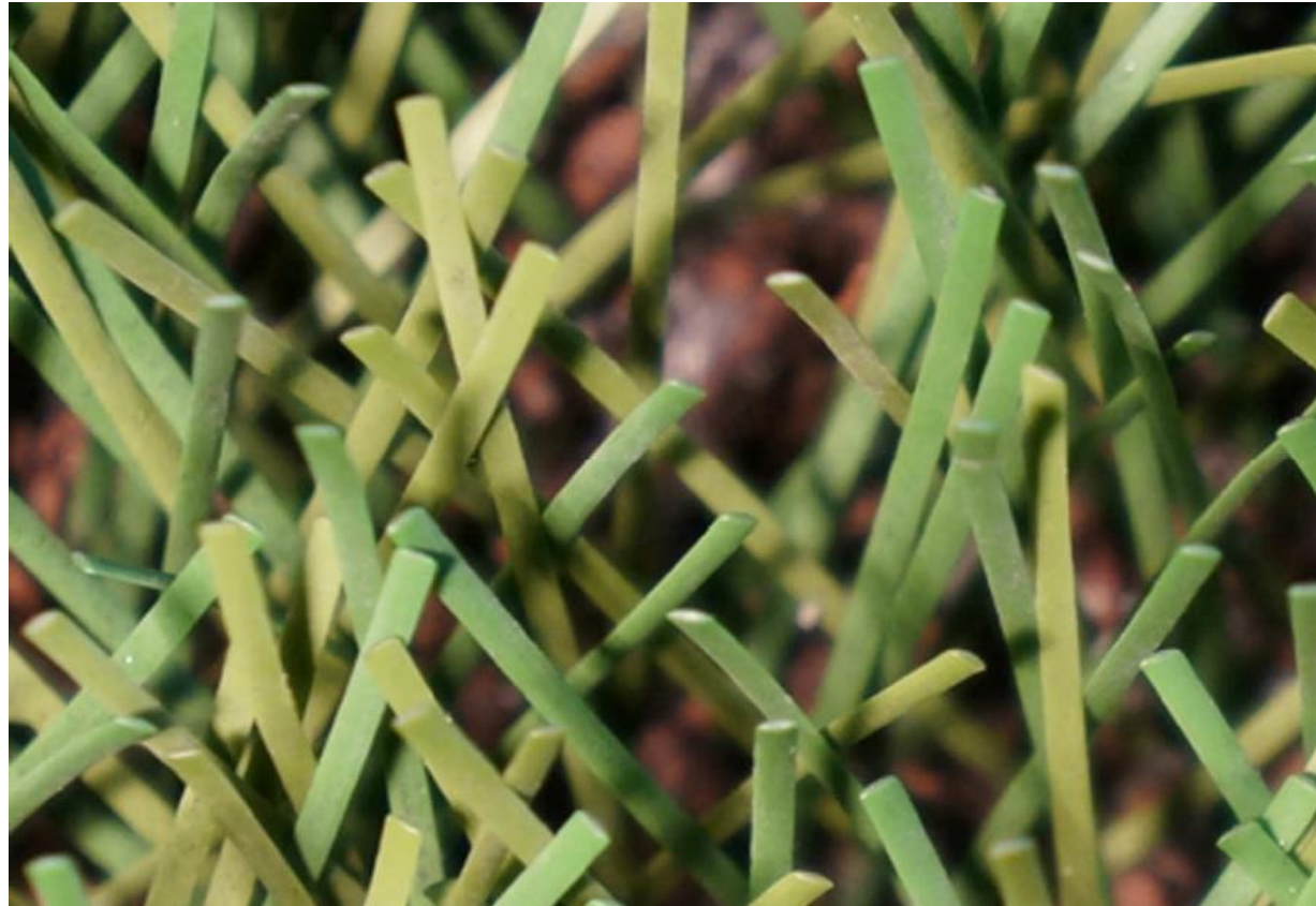
Fieldturf 360 after UV (DIN Spec) and 150 000 Cycles in a Lisport test (independent institute)
