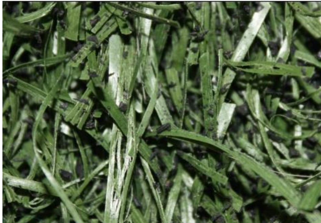
Competitor after 30 000 Cycles in the Lisport test, produced in USA
