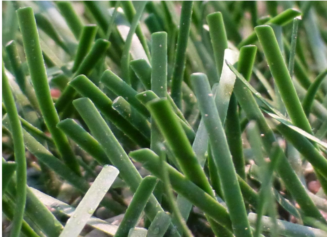
Fieldturf BiCo fiber (Core) after 200.000 Lysport cycles
