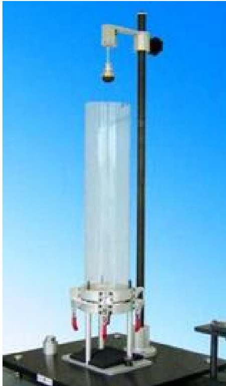
Dart drop test unit to measure energy Absorption of film
