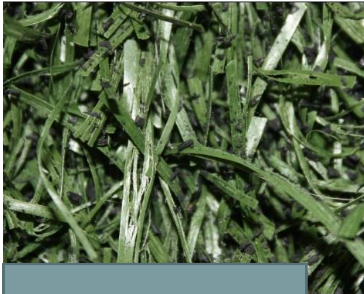
Fiber made form plastic bag raw material (1,04 " /m 2 )
