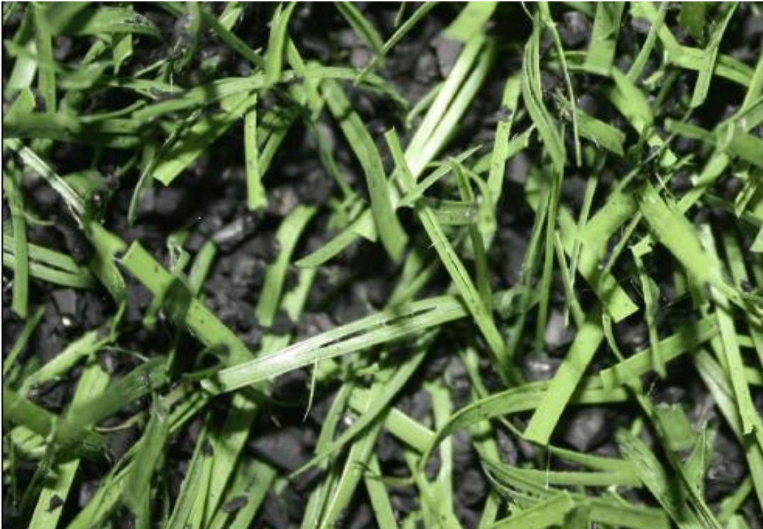
Competitor after 30 000 Cycles at Lisport test, Produced in the middle east
