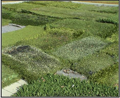
Between laboratory testing, yarns from site and yarns not exposed we noticed a loss in tensile properties and loss of abrasion resistance but also a loss in the melting point. We did the same for several damages and always found a correlation between site and lab exposure. I also noticed that good yarns never failed in the QUV, lamps B.
