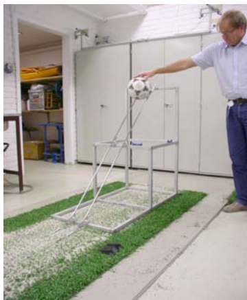
Photo 3 Timing gate for measuring velocity change
