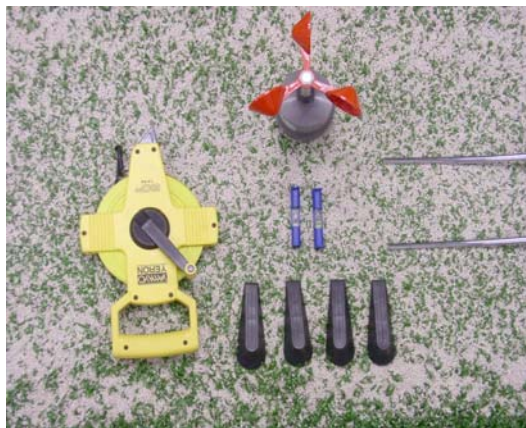
Photo 2: Wind speed sensor, steel tape and levelling device
