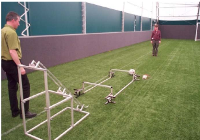
Photo 3 Timing gate for measuring velocity change
