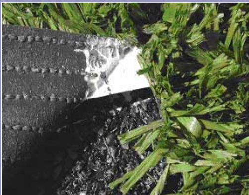
Turf joint: strong adhesion
