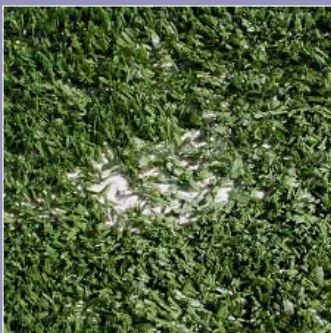
Stabilisation infill with quartz sand
