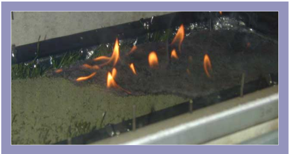
Flame test with a football turf
