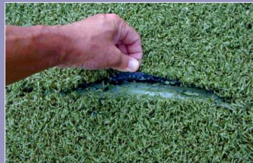
Torn seam joint
