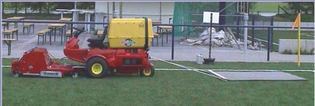
Brushing, aspiration, cleaning and levelling in one go.
